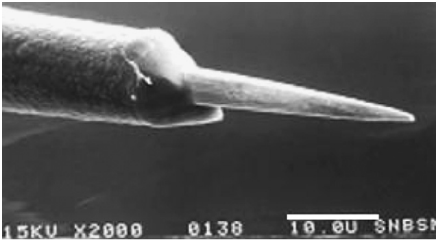
Fig. 2. An SEM of an electrode used in the FMA. This electrode was pre-treated with A-174 Silane before being insulated with 3 \mu\text{m} of Parylene-C. The tip was exposed by a non-thermal ablation technique using a dual beam Eximer Laser System having a wave length of 248 nm. This is an image of an arbitrary electrode that may not have been used in this study. Reprinted from Journal of Neuroscience Methods, 62, Schmidt, Bak and Christensen, Laser Ablation Paralyne-C insulated, 89–92, 1995, with permission from Elsevier.
